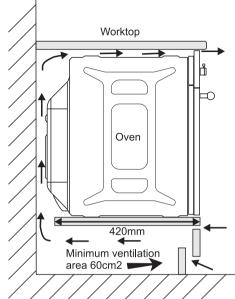
When placing the oven in the housing, do not use the oven door as a lever for lifting the oven as damage may result. Once the oven has been positioned in the housing it should be secured in place at the four corners of the oven doorframe using suitable screws (see diagram).
